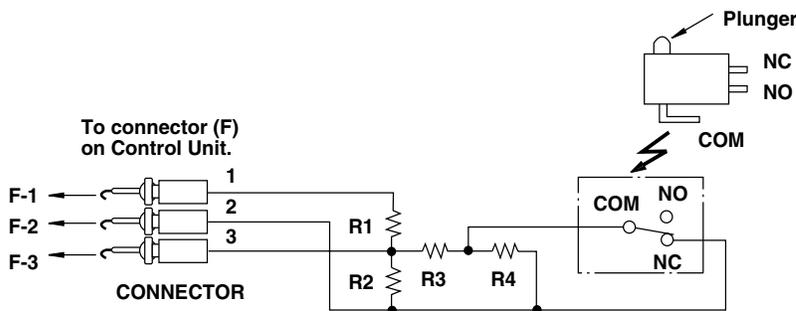
**Sensor Dummy Resistor Circuit**
