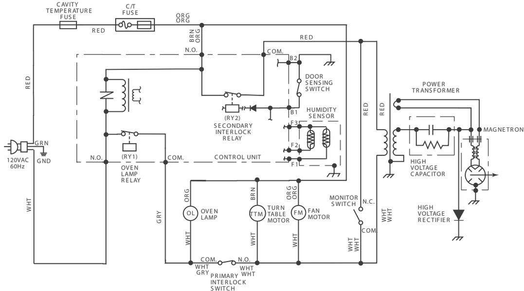
Figure O-2 Oven Schematic - Cooking Condition
