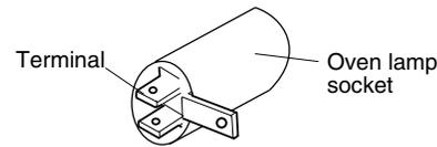
Figure C-1. Oven lamp socket
