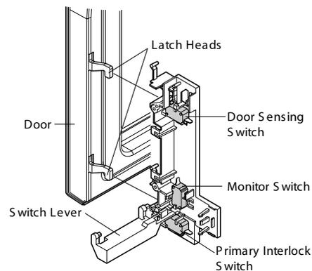
Figure C-3. Latch Switch Adjustments
